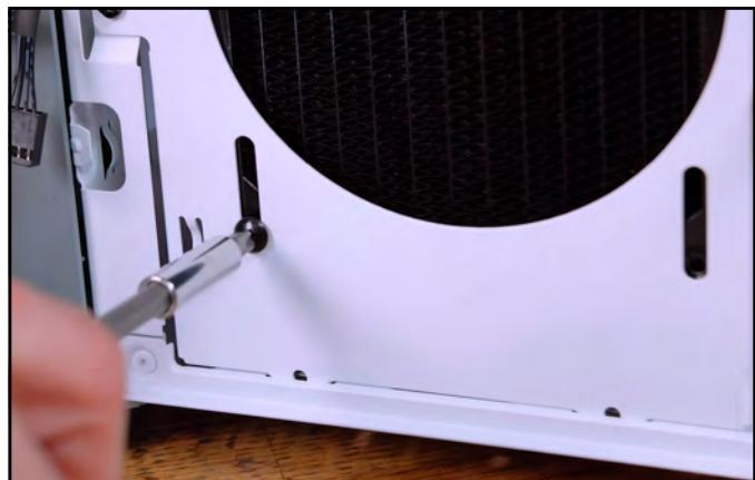
**B:** Used when mounting standard 25mm-thick fans to the radiator, either directly or through a chassis.
