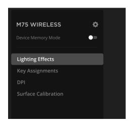
Device memory mode allows a product to utillized in iCUE in the 'hardware state'. Previous iterations of iCUE require you to quit iCUE in order for a device to work in the hardware state. Hardware states for our devices allow for device behavior without a dependency on iCUE running in the background. Examples of hardware states include the color of lighting on your Fans and Coolers under 'Hardware Lighting' or Hardware Key Assignments for your mouse and keyboard.
