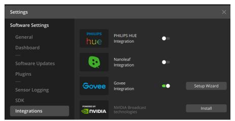
For proper setup of Govee devices with iCUE, please follow the Setup Wizard exactly as described. You will need to enable **LAN Control** in your Govee mobile application as a part of the setup process. The following products are supported in our initial beta of Govee support:
